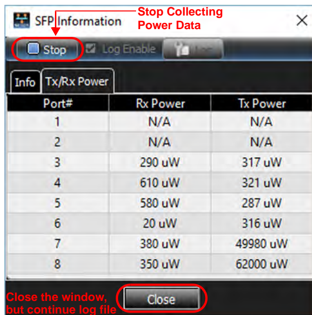
Figure 4.43: Tx/Rx Power Being Logged
